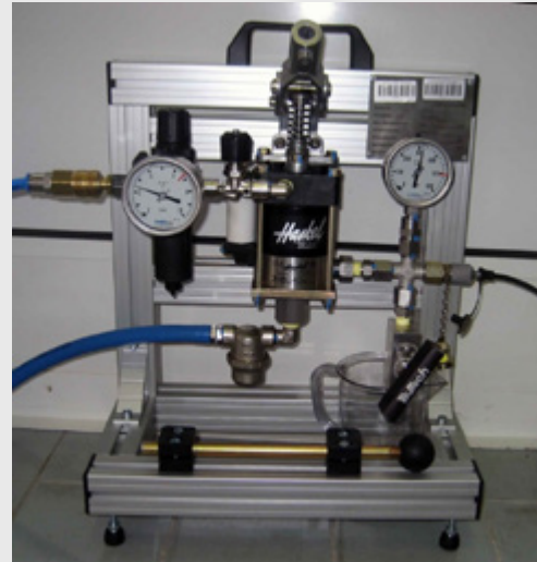
Figure 7: The pressure booster (make: Haskel) used for the tests
